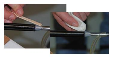
7. Once the epoxy has cured, begin to wrap from the shaft of the hook up onto the blank with thread (run thread at least half the length of the shaft) this helps to strengthen the blank.
